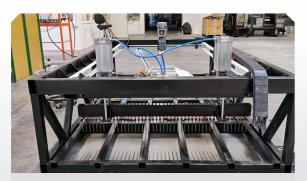
Naked WindowBuster™ before mounting body and electrical cabinet. ~600kg.
